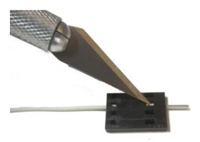
After removing the pin, lift the lever of the pin back up so that it will lock itself when placed back in the housing.
