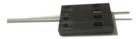
To remove the pin, push the lever of the pin to allow the pin to slide out of the black housing.
